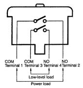
Note: The circuit switching power load has a snap-action mechanism.
