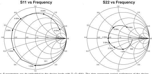
Note: S-parameters are de-embedded to the device leads with  $Z_s = Z_L = 50\Omega$ . The data represents typical performace of the device. De-embedded s-parameters can be downloaded from our website (www.sirenza.com).
