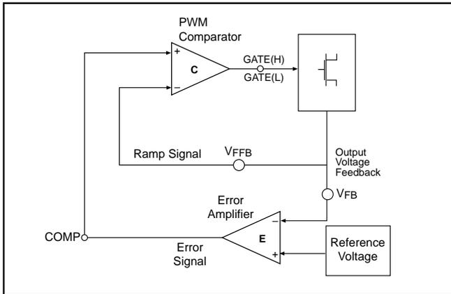
Figure 1: V<sup>2</sup>™ Control Diagram.
