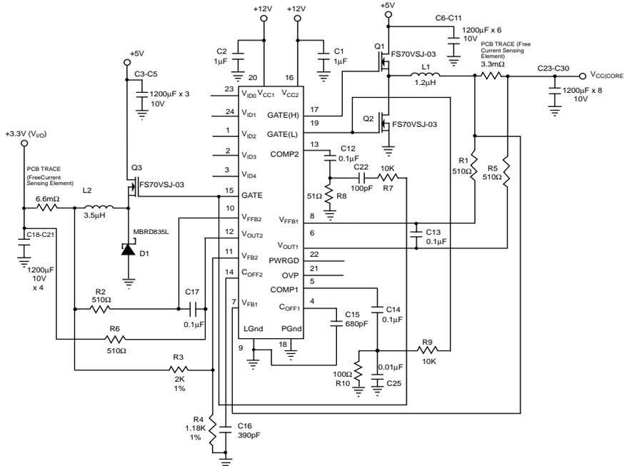
5V/12V to 2V/16A for Pentium® II V<sub>CC(CORE)</sub>, 5V/12V to 3.3V/8A for V<sub>I/O</sub>
