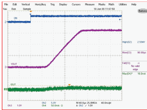
Figure 26. Turn-On Response (V_{IN}=3.3V, C_{IN}=1\mu F, C_{OUT}=0.1\mu F, R_L=500\Omega)
