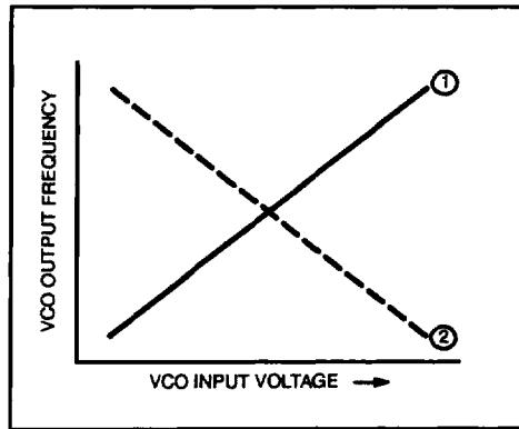
Depending upon VCO polarity, FC pin should be set accordingly:
