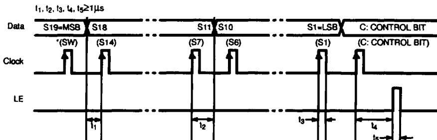
NOTES: Parenthesis data is used for setting divide ratio of programmable reference divider.
