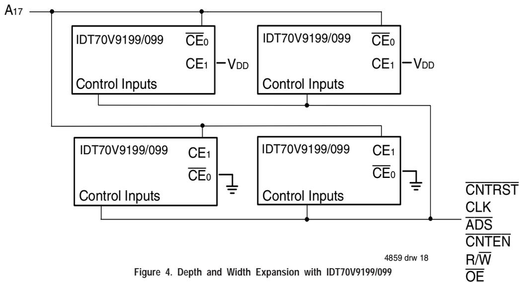
Figure 4. Depth and Width Expansion with IDT70V9199/099
