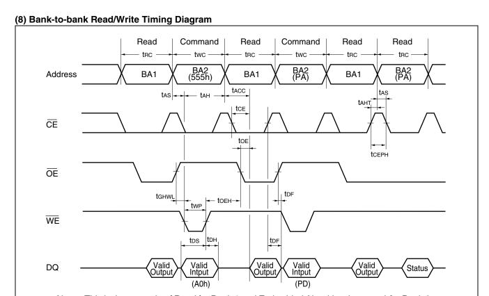
Note: This is the example of Read for Bank 1 and Embedded Algorithm (program) for Bank 2. BA1: Address corresponding to Bank 1. BA2: Address corresponding to Bank 2.
