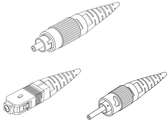
Epoxy and Polish ST® Compatible, FC, and SC Connectors | Drawing ZA-1055
