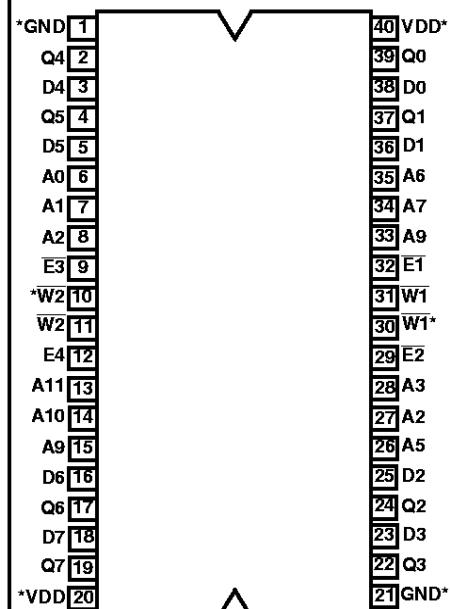
\* Pins 20 and 40 (VDD) are internally connected. Similarly pins 1 and 21 (Ground) are connected. The user is advised to connect both VDD pins and both Ground pins to the board busses. This will improve power distribution across the array and will enhance decoupling.
