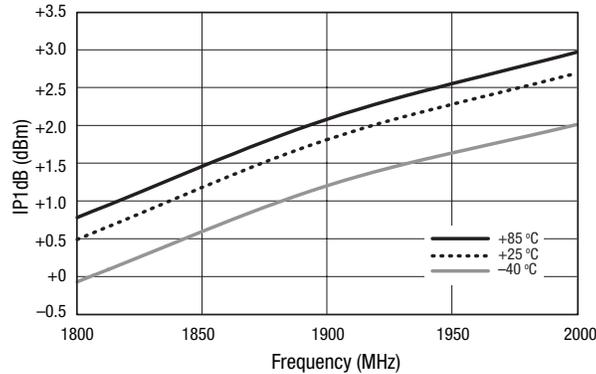
Figure 16. IP1dB vs Frequency Over Temperature
