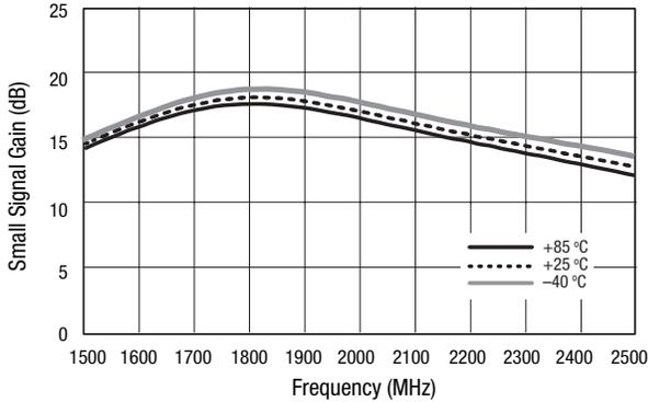
**Figure 10. Small Signal Gain vs Frequency Over Temperature,  $P_{IN} = -20\ \text{dBm}$**
