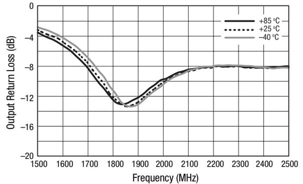
**Figure 13. Output Return Loss vs Frequency Over Temperatures,  $P_{IN} = -20\ \text{dBm}$**
