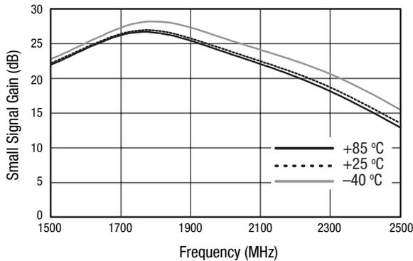
**Figure 4. Small Signal Gain vs Frequency Over Temperature, P<sub>IN</sub> = -20 dBm**
