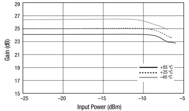
**Figure 9. Gain vs Input Power Over Temperature,  $f = 1950$  MHz**
