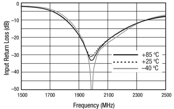
**Figure 5. Input Return Loss vs Frequency Over Temperature, P<sub>IN</sub> = -20 dBm**
