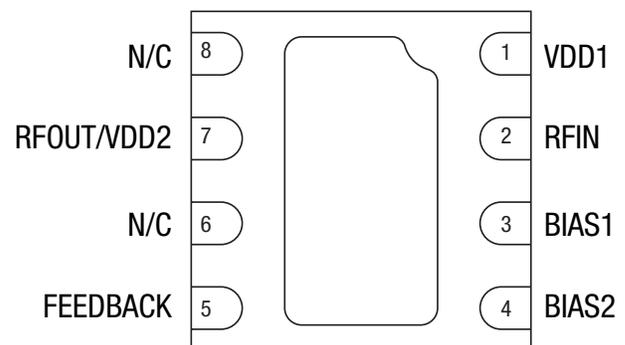
**Figure 2. SKY65040-360LF Pinout – 8-Pin QFN (Bottom View)**
