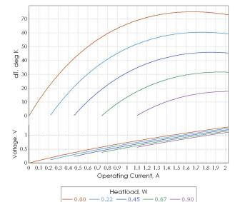
**Note**: Performance data is specified for optimal optimal conditions (TEC hot side is stabilized at ambient temperature). Heatsink thermal resistance is not included into estimations. Use TECCad Software for estimations under different conditions.
