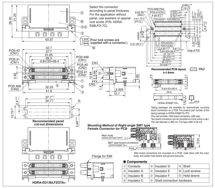
Mating connector: HDRA series IDC type male cable connector, or straddle SMT type male connector
