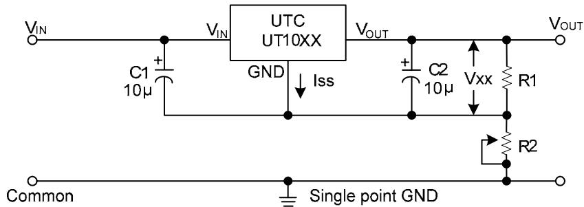
$$V_{OUT} = V_{xx}(1 + \frac{R2}{R1}) + I_{ss}R2$$
