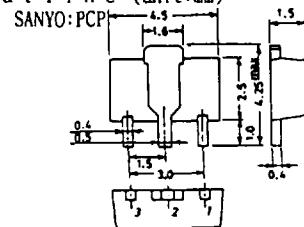
For PNP, (-) sign is omitted. PC : Mounted on ceramic board(250mm<sup>2</sup>×0.8mm).
