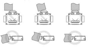
Do not operate the plunger from the side. Doing so may deform or damage the Switch.
