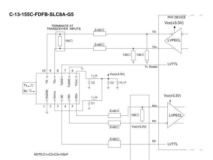
The split-loaded terminations for ECL signals need to be located at the input of devices receiving those ECL signals.
