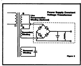
**Power Supply Constant Voltage Transformer:** This type of transformer has a quasi-square wave output making it ideal for rectified output circuits.
