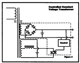
**Controlled Constant Voltage Transformer:** This type of transformer employs a separate external feedback circuit to provide tighter regulation for line, load, frequency, and temperature variations.
