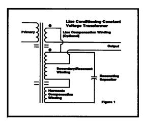
**Line Conditioning Constant Voltage:** The output of this type of transformer is regulated to relatively constant output voltage and is constructed in such a manner that the harmonic content is relatively low making it ideal for most electronic equipment.
