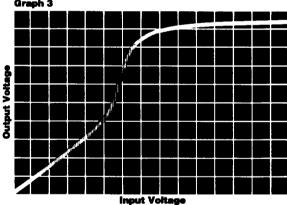
**Regulation:** The change in output voltage for given changes of input voltage, output load, power factor, frequency or any combinations, expressed in percent.
