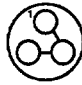
Three (3) Size 16 Contacts 0.063 inch (1.6 mm) Minimum Creepage for Operation at 300V RMS
