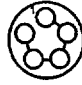
Five (5) Size 20 Contacts 0.039 inch (1.0 mm) Minimum Creepage for Operation at 200V RMS
