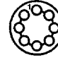
Eight (8) Size 22 Contacts 0.028 inch (0.7 mm) Minimum Creepage for Operation at 100V RMS
