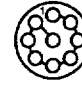
Nine (9) Size 22 Contacts 0.028 inch (0.7 mm) Minimum Creepage for Operation at 100V RMS
