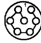
Seven (7) Size 22 Contacts 0.063 inch (1.6 mm) Minimum Creepage for Operation at 300V RMS
