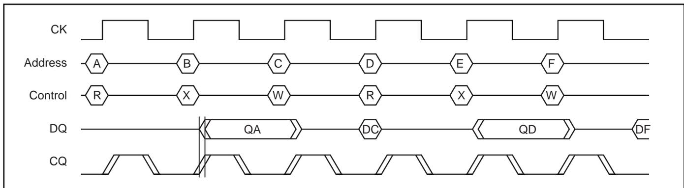
**DOUBLE DATA RATE WRITE—DOUBLE DATA RATE READ ( $\Sigma 1 \times 2Lp$ ). For reference only.**
