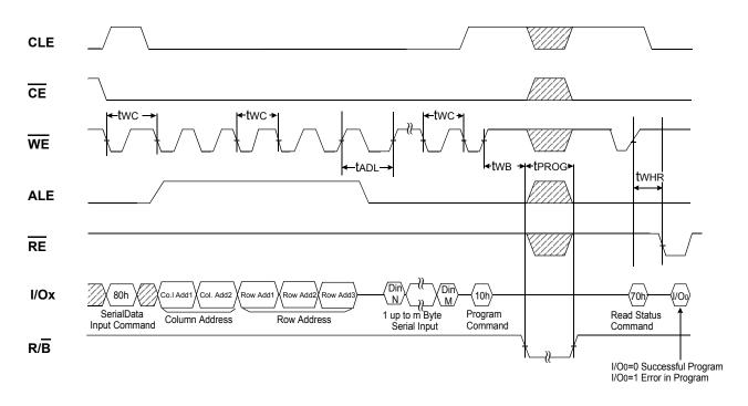
NOTES : tADL is the time from the  $\overline{WE}$  rising edge of final address cycle to the  $\overline{WE}$  rising edge of first data cycle.
