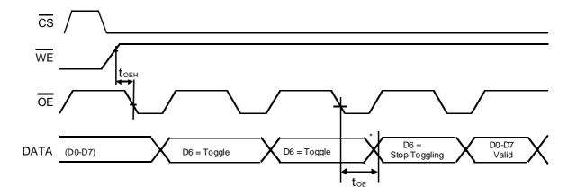
\* D6 stops toggling (the device has completed the embedded operations)
