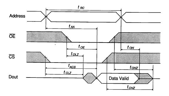
t<sub>Hz</sub> and t<sub>OHz</sub> are defined as the time at which the outputs achieve open circuit conditions and are not referenced to output voltage levels. These parameters are sampled and not 100% tested.
