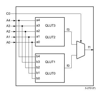
Figure 8. F5M Mode—One Six-Input Variable Function
