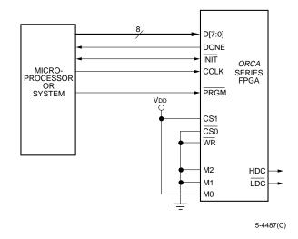
Figure 46. Slave Parallel Configuration Schematic
