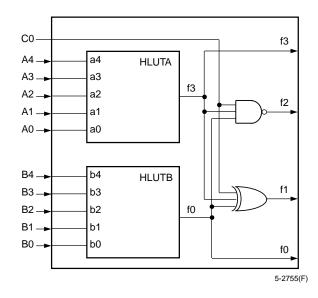
Figure 7. F5X Mode—Exclusive OR Function of Two Independent Five-Input Variable Functions
