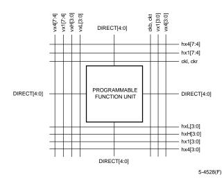
Figure 21. Single PLC View of Inter-PLC R-Nodes
