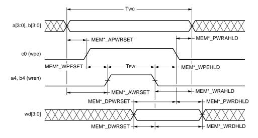
Figure 58. Write Operation
