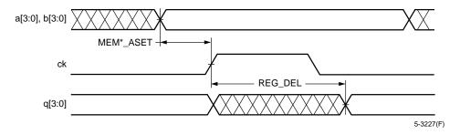
Figure 57. Read Operation—LUT Memory Loading Flip-Flops
