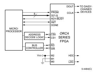
Figure 43. Asynchronous Peripheral Configuration Schematic
