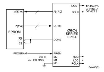
Figure 41. Master Parallel Configuration Schematic
