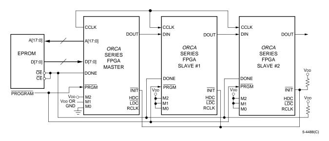
Figure 47. Daisy-Chain Configuration Schematic
