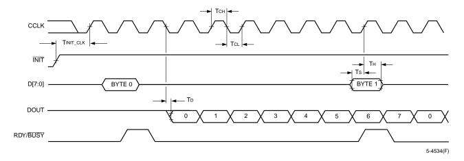
Figure 70. Synchronous Peripheral Configuration Mode Timing Diagram
