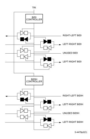
Figure 20. 3-Statable Bidirectional Buffers
