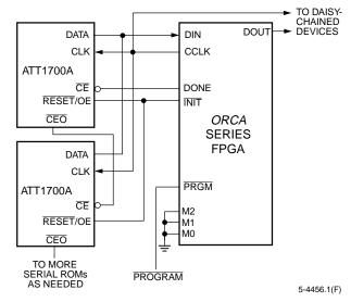
Figure 42. Master Serial Configuration Schematic
