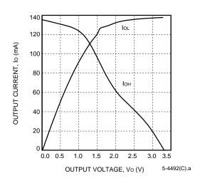
Figure 85. Slewlim (TJ = 25  $^{\circ}$ C, VDD = 3.3 V)
