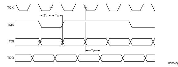
Figure 74. Boundary-Scan Timing Diagram
