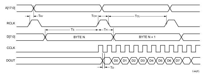
Figure 68. Master Parallel Configuration Mode Timing Diagram
