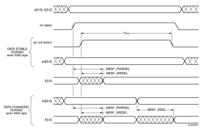
Figure 59. Read During Write
