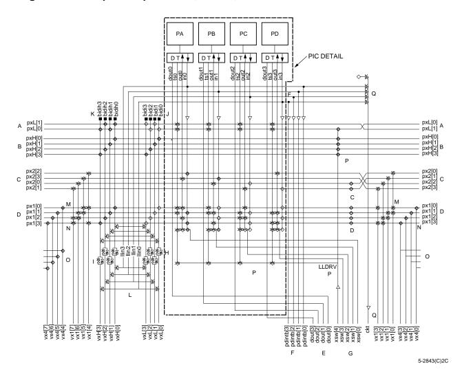
Figure 26. PIC Architecture
