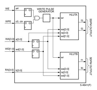
Figure 17. SDPM Mode—16 x 2 Synchronous Dual-Port Memory
