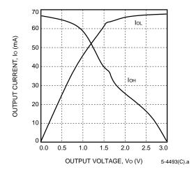
Figure 88. Slewlim (T<sub>J</sub> = 125  $^{\circ}$ C, V<sub>DD</sub> = 3.0 V)
