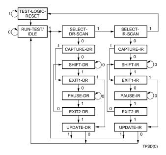
Figure 51. TAP Controller State Transition Diagram
