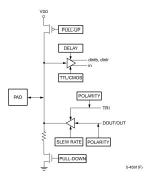
Figure 24A. Simplified Diagram of OR2CxxA
