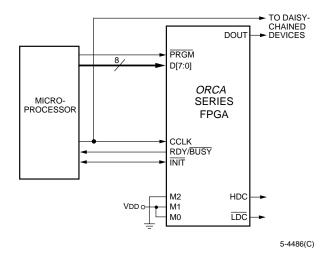
Figure 44. Synchronous Peripheral Configuration Schematic
