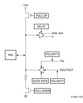
Figure 24B. Simplified Diagram of OR2TxxA
