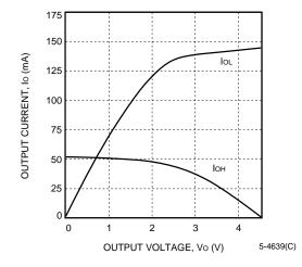
Figure 83. Fast (TJ = 125  $^{\circ}$ C, VDD = 4.5 V)
