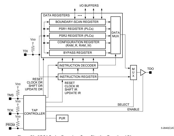
Figure 50. ORCA Series Boundary-Scan Circuitry Functional Diagram
