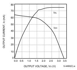
Figure 84. Sinklim (TJ = 25  $^{\circ}$ C, VDD = 3.3 V)
