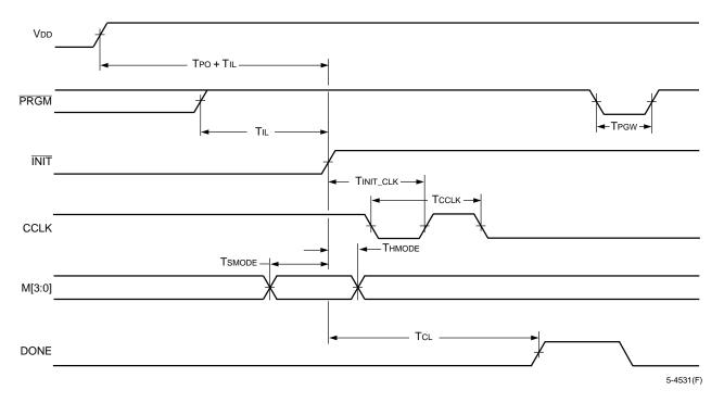
Figure 66. General Configuration Mode Timing Diagram
