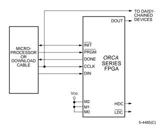
Figure 45. Slave Serial Configuration Schematic
