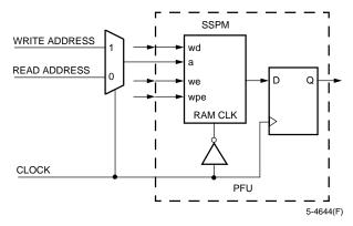
Figure 15. SSPM with Read/Write per Clock Cycle
