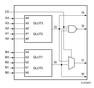
Figure 6. F5M Mode—Multiplexed Function of Two Independent Five-Input Variable Functions
