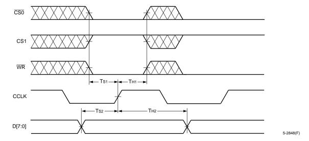
Figure 72. Slave Parallel Configuration Mode Timing Diagram
