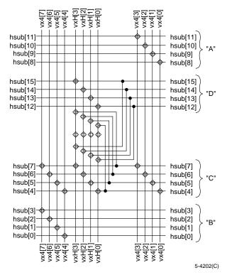
Figure 32. Horizontal Subquad Routing Connectivity (Half Quad)
