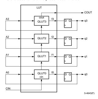
Figure 10. Counter Submode with Flip-Flops
