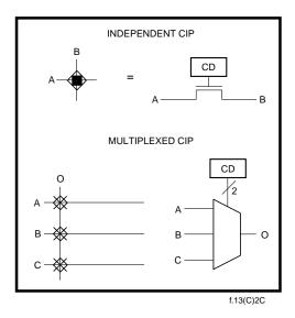
Figure 19. Configurable Interconnect Point
