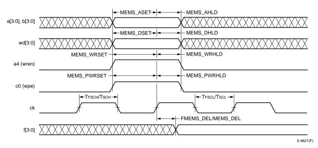
Figure 61. Synchronous Memory Write Characteristics
