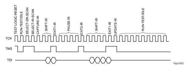
Figure 53. Instruction Register Scan Timing Diagram
