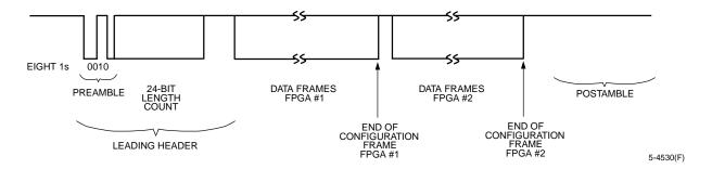
Figure 39. Serial Configuration Data Format
