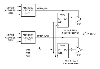
Note: The lower address bits are not shown.
