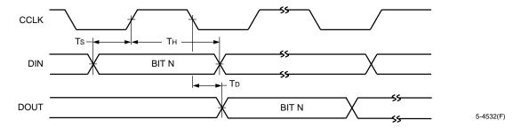
Figure 67. Master Serial Configuration Mode Timing Diagram
