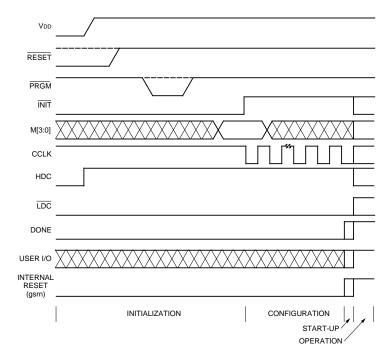
Figure 37. Initialization/Configuration/Start-Up Waveforms
