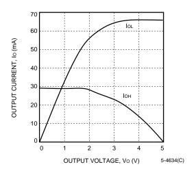
Figure 78. Sinklim (TJ = 25  $^{\circ}$ C, VDD = 5.0 V)
