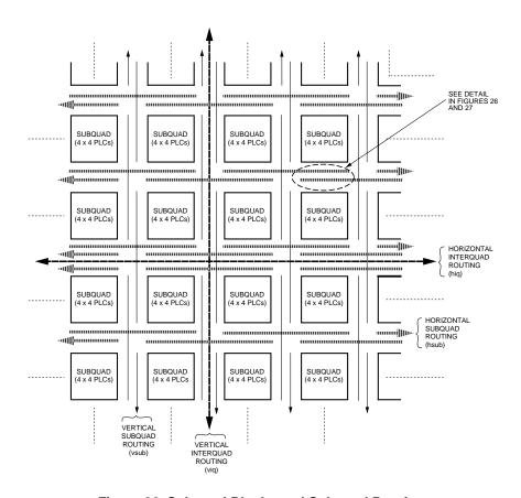
Figure 30. Subquad Blocks and Subquad Routing
