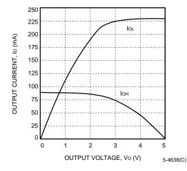
Figure 80. Fast (TJ = 25  $^{\circ}$ C, VDD = 5.0 V)
