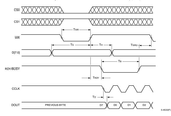
Figure 69. Asynchronous Peripheral Configuration Mode Timing Diagram
