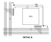
Figure 35. Secondary Clock Distribution
