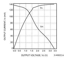
Figure 86. Fast (TJ = 25  $^{\circ}$ C, VDD = 3.3 V)
