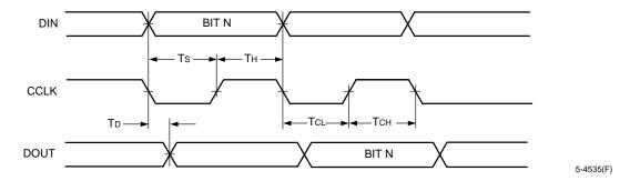
Figure 71. Slave Serial Configuration Mode Timing Diagram
