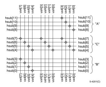
Figure 31. Horizontal Subquad Routing Connectivity
