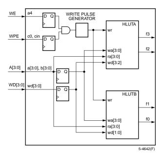
Figure 14. SSPM Mode—16 x 4 Synchronous Single-Port Memory
