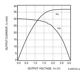
Figure 87. Sinklim (TJ = 125  $^{\circ}$ C, VDD = 3.0 V)
