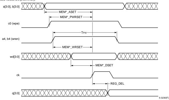
Figure 60. Read During Write—Clocking Data into Flip-Flop
