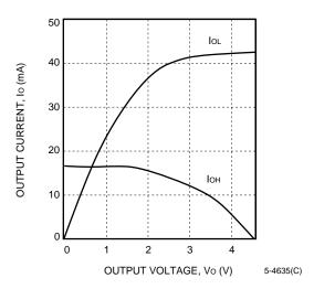
Figure 81. Sinklim (TJ = 125  $^{\circ}$ C, VDD = 4.5 V)
