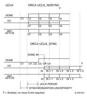
Figure 38. Start-Up Waveforms
