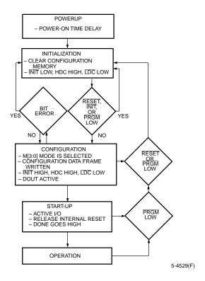
Figure 36. FPGA States of Operation
