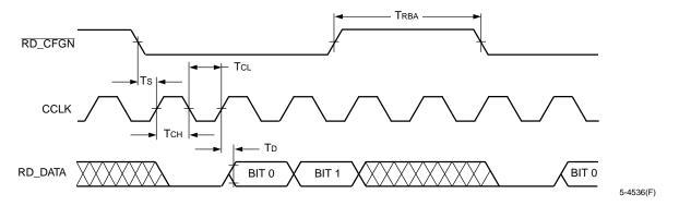
Figure 73. Readback Timing Diagram
