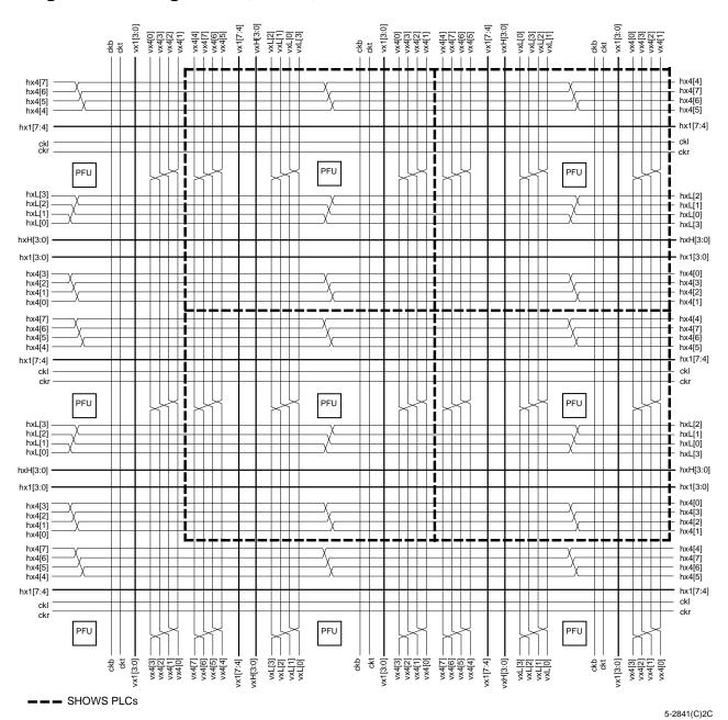
Figure 22. Multiple PLC View of Inter-PLC Routing
