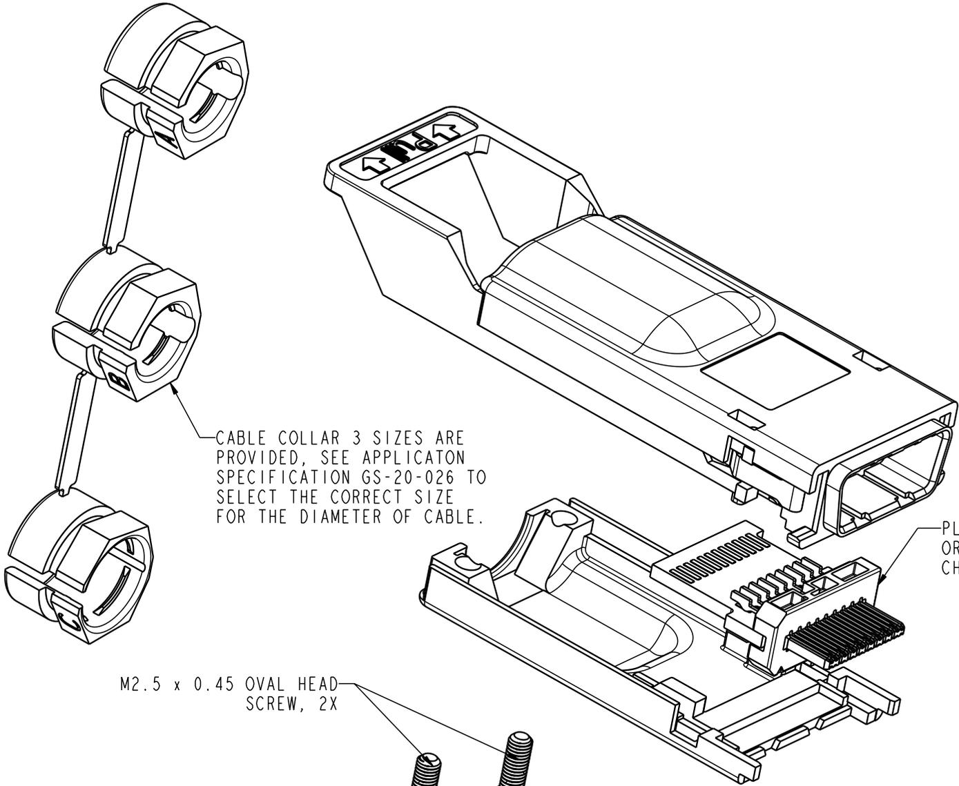
CABLE COLLAR 3 SIZES ARE PROVIDED, SEE APPLICATION SPECIFICATION GS-20-026 TO SELECT THE CORRECT SIZE FOR THE DIAMETER OF CABLE.
