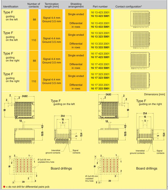
Thin print part numbers:0.76 μm (30 μinch) Gold on contact area= performance level 1Bold print part numbers:Gold flash over 1.02 μm (40 μinch) Palladium-Nickel on contact area= performance level 2\* Additional information see page 3
