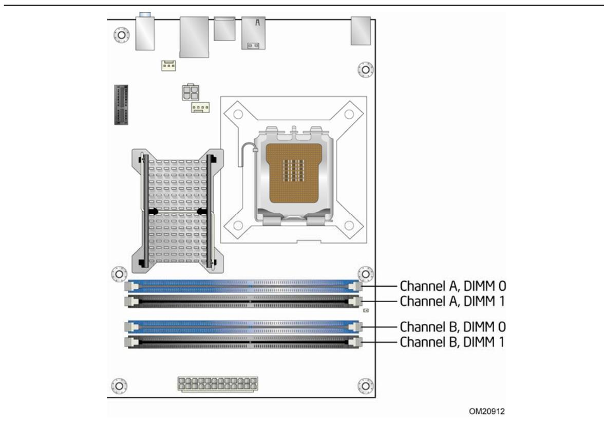
**Figure 3. Memory Channel Configuration and DIMM Configuration**
