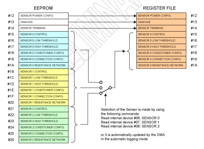
The configuration of the selected sensor is automatically loaded from EEPROM when:
