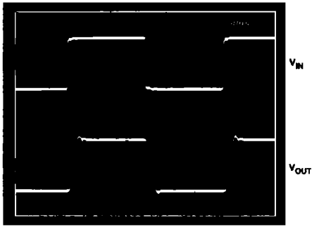
Figure 25. Large Signal Pulse Response, Gain = +10, ( R_F = 357 \Omega , R_L = 500 \Omega , V_S = \pm 15 V )
