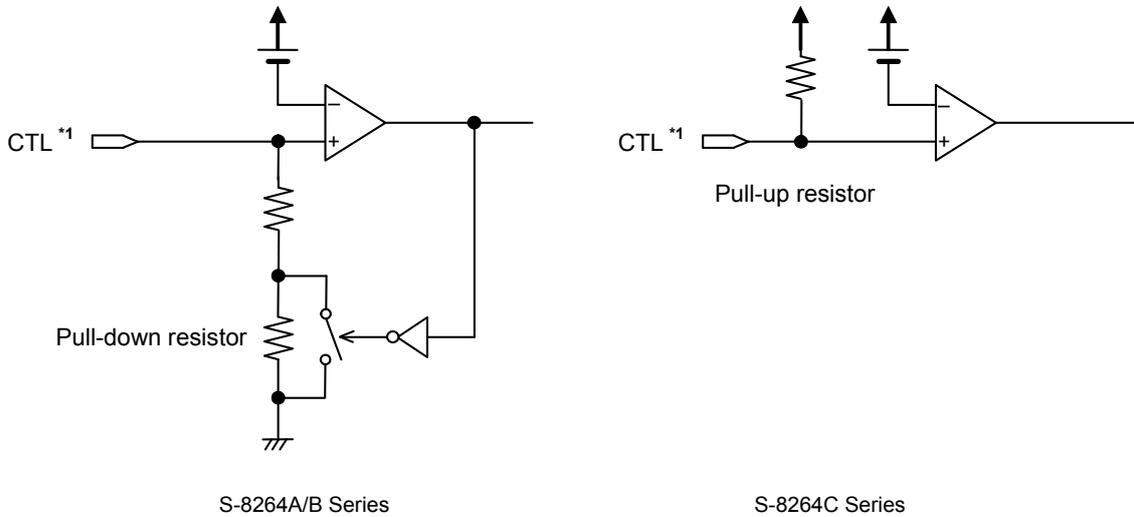
\*1. The reverse voltage “H” to “L” or “L” to “H” of CTL pin is VDD pin voltage – 2.8 V (Typ.), does not have the hysteresis.
