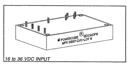
Powercube's 15 watt **Dual Output Micro-Series** modules are rugged, low profile, current mode control switching regulators providing fully isolated, efficient power conversion from a broad DC input range. These units are parallelable and load share within five percent. Outputs may also be connected in series and trimmed to provide higher voltages. They also include overload and short circuit protection, overvoltage protection by zener diode, and on/off control.
