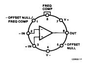
Lead 4 connected to case.
