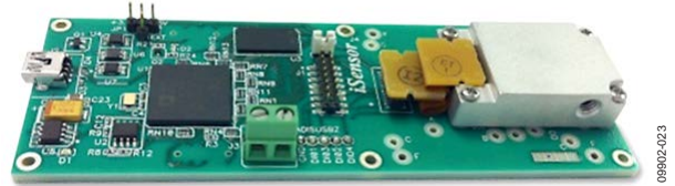
Figure 3. ADIS16448/PCBZ Installation Example
