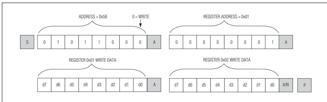
Figure 10. Format for Writing to Multiple Registers
