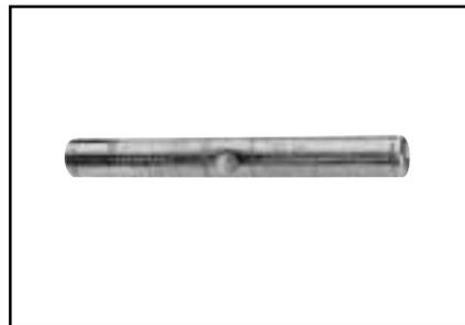
Full-tension HYSPLICE™ sleeves designed for HS, EHS, Utilities (UT) or Siemens-Martin (SM) galvanized steel guy, messenger, and "Static" conductors. Made of hot-dip galvanized seamless milled steel tubing lined with silicone carbide particles.
