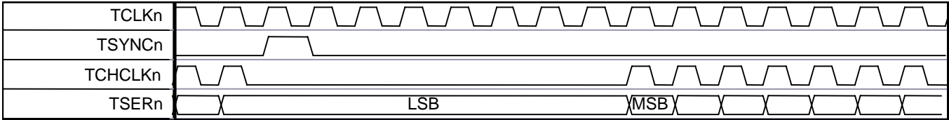
Figure 11-31. E1 Transmit-Side TCHCLKn Gapped Mode During Channel 1
