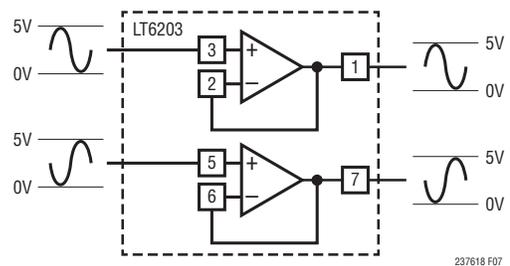
Figure 7. LT6203 Buffering a Fully Differential Signal Source
