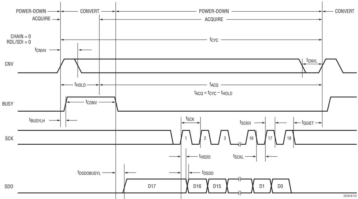
Figure 13. Using a Single LTC2376-18 in Normal Mode
