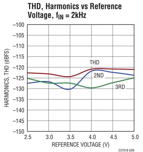
**TYPICAL PERFORMANCE CHARACTERISTICS**  $T_A = 25^\circ\text{C}$ ,  $V_{DD} = 2.5\text{V}$ ,  $0V_{DD} = 2.5\text{V}$ ,  $V_{CM} = 2.5\text{V}$ ,
