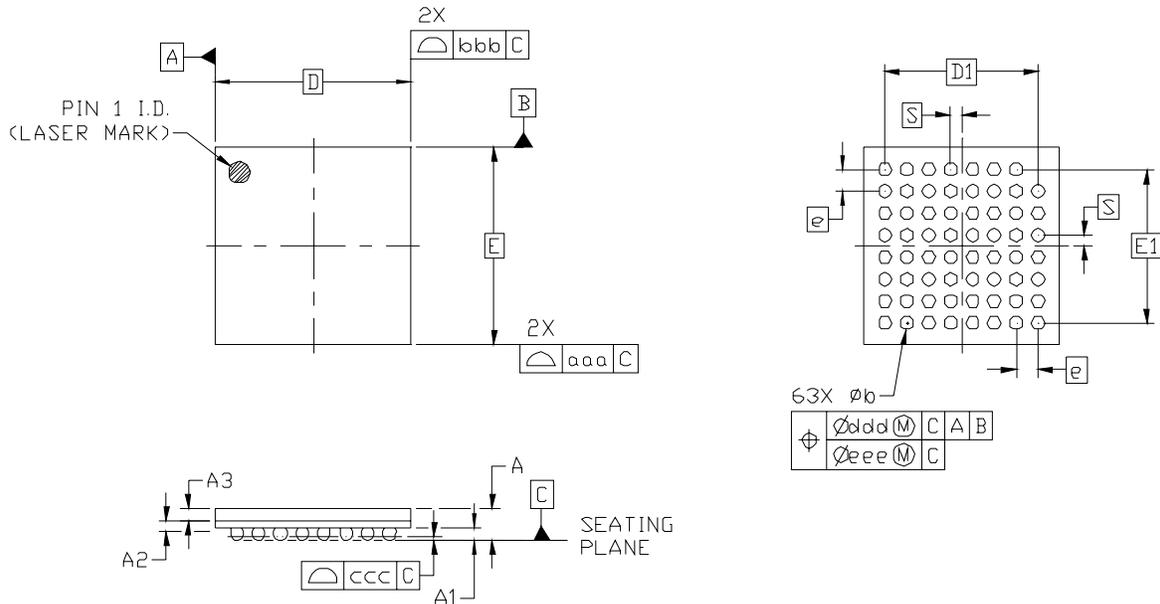
**Figure 14. 63-Ball Plastic Ball Grid Array (PBGA)**
