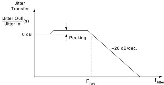
**Figure 7. PLL Jitter Transfer Mask/Template**
