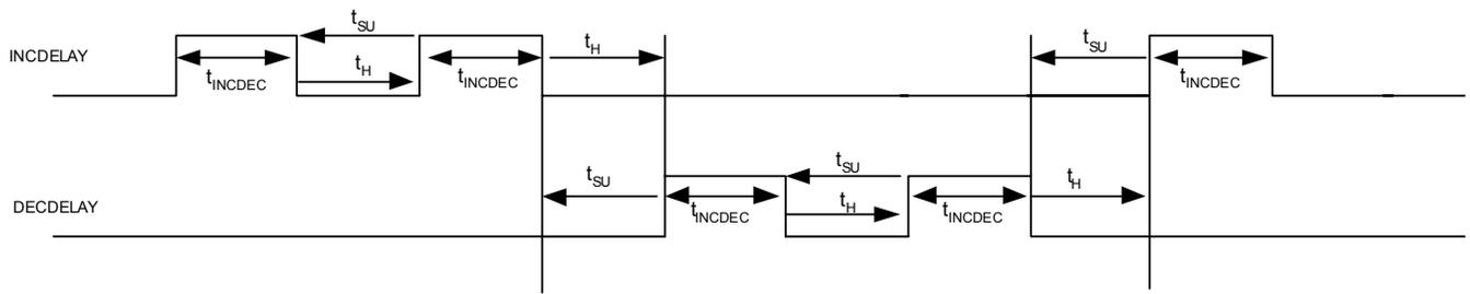
**Figure 4. Output Phase Adjust Timing Diagrams (Pin Control)**
