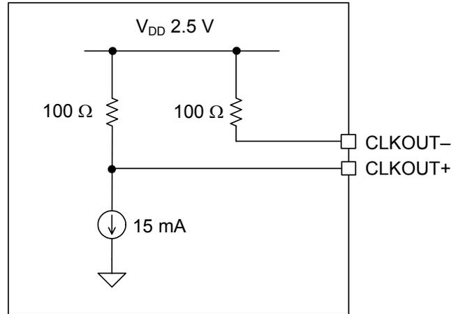
**Figure 10. CLKOUT± Equivalent Circuit, RSTN/CAL Asserted LOW**
