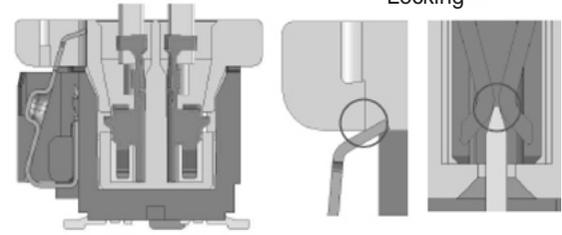
A clear click engagement generated when locking starts, matching that of the terminal which comes into contact.
