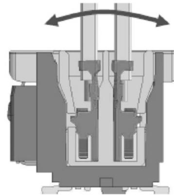
A structure that withstands stresses with deep mating. The thick external wall enhances strength against wall breakage.
