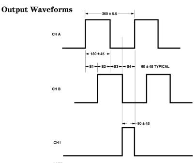
NOTE: ALL VALUES ARE IN ELECTRICAL DEGREES, WHERE 360° e = 1 CYCLE OF RESOLUTION. ERRORS ARE WORST CASE OVER ONE REVOLUTION. CH B LEADS CH A FOR COUNTERCLOCKWISE ROTATION. CH A LEADS CH B FOR CLOCKWISE ROTATION.
