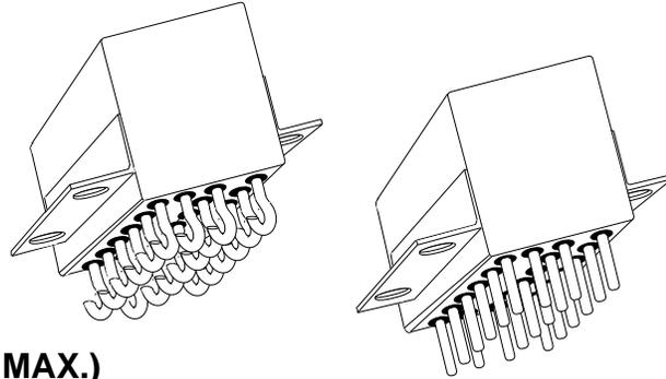
The Series FCA-610 relay is a polarized single-side stable design, where the flux from a permanent magnet provides the armature holding force in the deactivated state, and its flux path is switched and combined with the coil flux in the operated state. This results in appreciably increased contact pressure in both states over that of a spring return nonpolar design. We also manufacture 2-pole and 4-pole versions of this relay.
