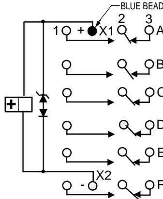
AC COILS (SOCKET PINS)
