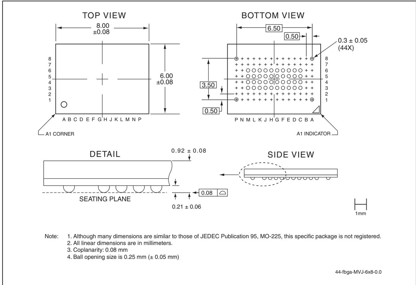
**FIGURE 27: 44-Ball Very Fine-pitch Ball Grid Array (VFBGA) 6mm x 8mm
