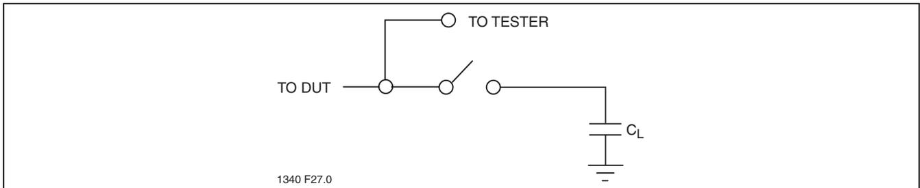
**FIGURE 21: A Test Load Example**
