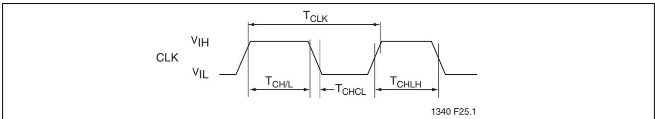
FIGURE 19: Clock Input AC Waveform
