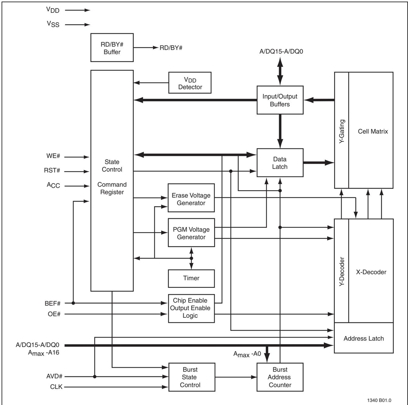
FIGURE 2: Logic Diagram
