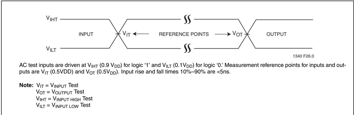
**FIGURE 20: AC Input/Output Reference Waveforms**
