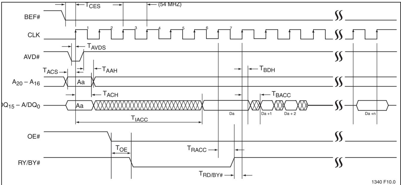
**Note:** Figure assumes seven wait states for initial access, 54 MHz clock, and automatic detect synchronous read. d0-d7 in data waveform indicate the order of data within a given 8-word address range, from lowest to highest. Data will wrap around within the 8 words, non-stop unless the RESET# is asserted low, or AVD# locks in another address. The device will output RD/BY# with valid data.
