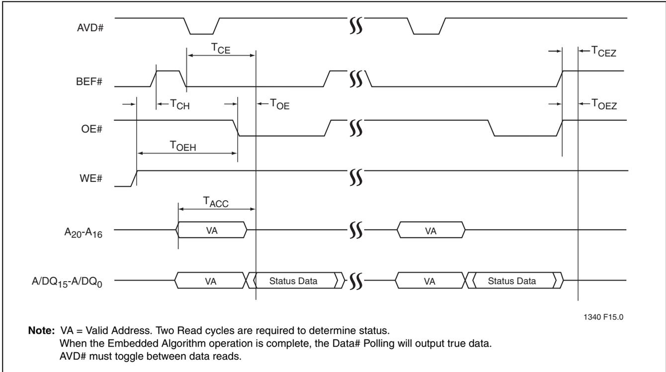
**FIGURE 12: Toggle Bit Timings (During Embedded Algorithms)**
