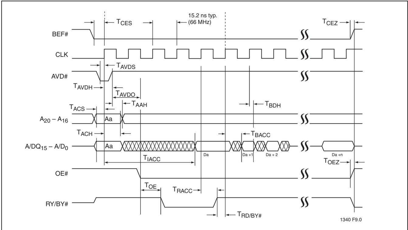
**FIGURE 5: CLK Synchronous Burst Mode Read**
