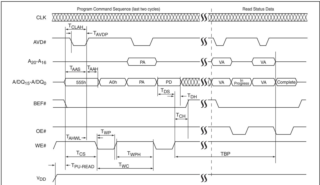
**Note:** PA= Program Address, PD = Program Data, VA = Valid Address for reading status bits.
