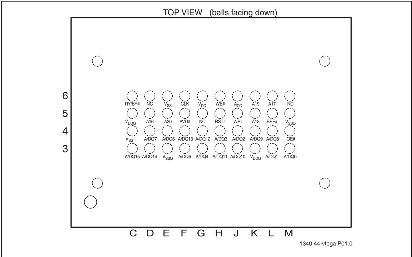
**FIGURE 3: Pin Assignments for 44-ball FBGA (6 x 8 mm)**
