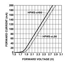
Figure 2. Forward Current vs. Forward Voltage.
