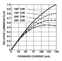
Figure 4. HPWS-xx00 Relative Luminous Flux vs. Forward Current.
