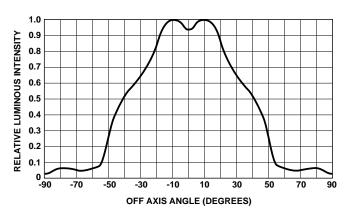
Figure 6a. HPWS-Tx00 Relative Intensity vs. Off Axis Angle.
