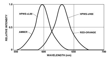
Figure 1. Relative Intensity vs. Wavelength.
