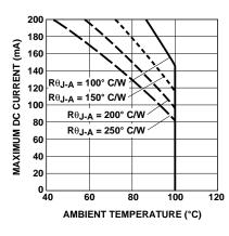
Figure 3b. HPWS-xx00 Maximum Pulsed Forward Current vs. Ambient Temperature.
