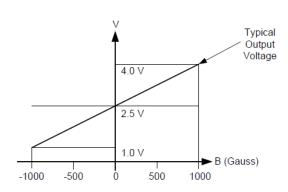
obtained with a supply voltage of 6V, but at the cost of increased supply current and a slight loss of output symmetry. So, it is not recommended to work in such condition unless the output voltage magnitude is a main issue. The output signal can be capacitively coupled to an amplifier for boosting further if the changing frequency of the magnetic field is high.
