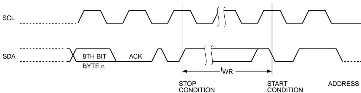
**Figure 3. Start/Stop Timing**
