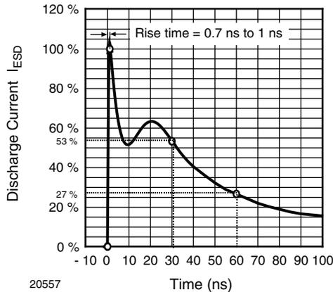
Fig. 1 - ESD Discharge Current Wave Form
