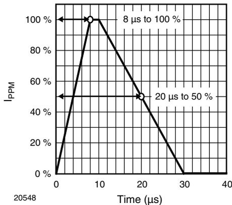
Fig. 2 - 8/20 μs Peak Pulse Current Wave Form
