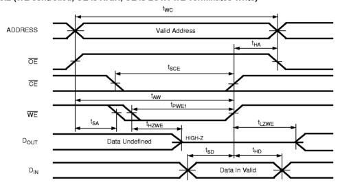
Write Cycle No.3 ( $\overline{\text{WE}}$  controlled,  $\overline{\text{OE}}$  is LOW;  $\overline{\text{CE}}$  is LOW:  $\overline{\text{WE}}$  Terminates Write) <sup>10</sup>
