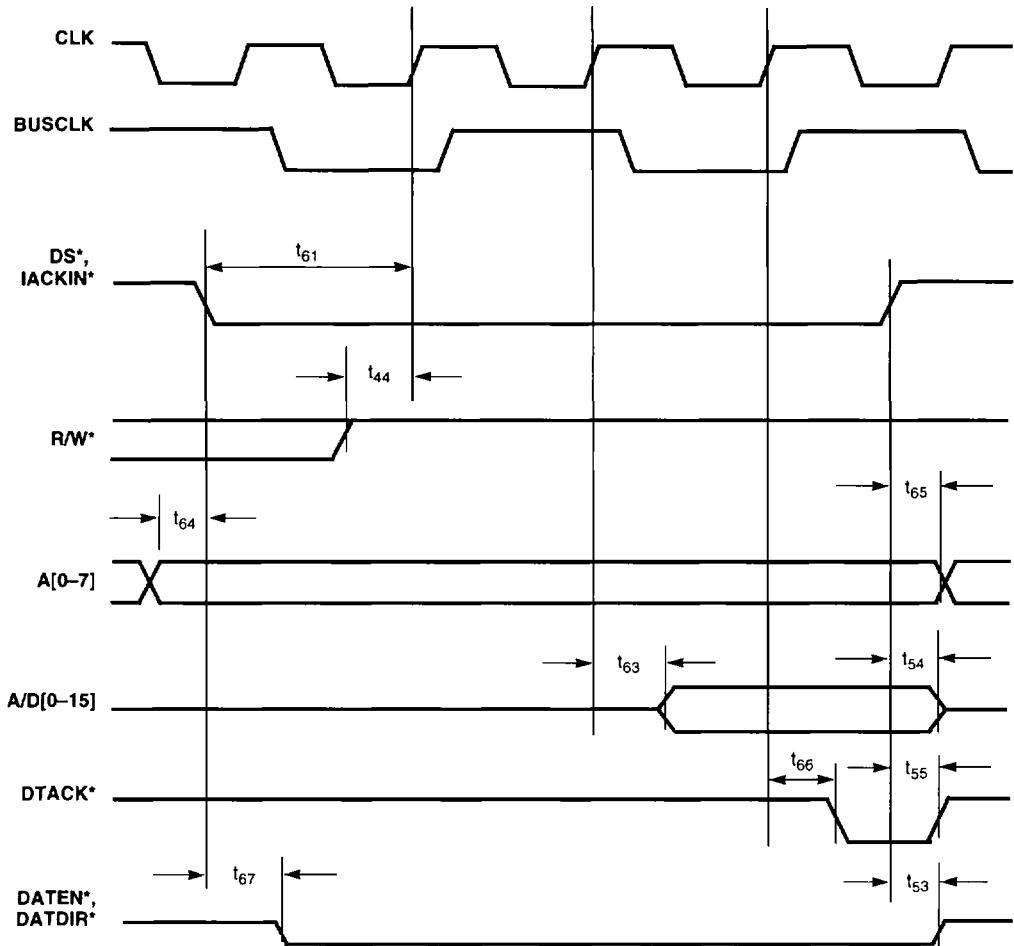
**Figure 7-3. Interrupt Acknowledge Cycle Timing**
