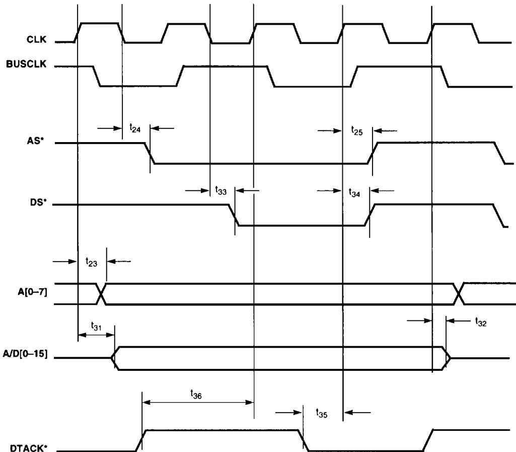
Figure 7-7. DMA Write Cycle Timing
