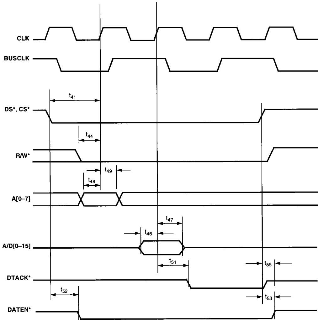
**Figure 7-2. Slave Write Cycle Timing**
