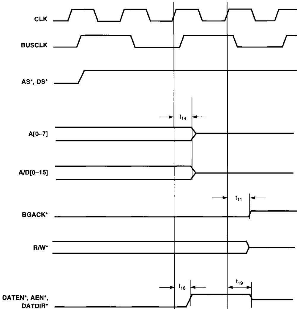
**Figure 7-5. Bus Release Timing**
