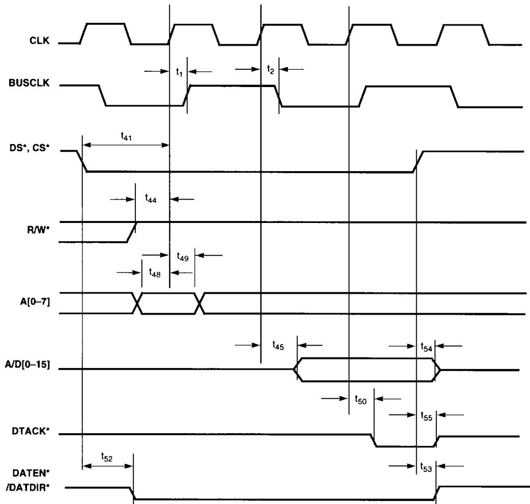
Figure 7-1. Slave Read Cycle Timing
