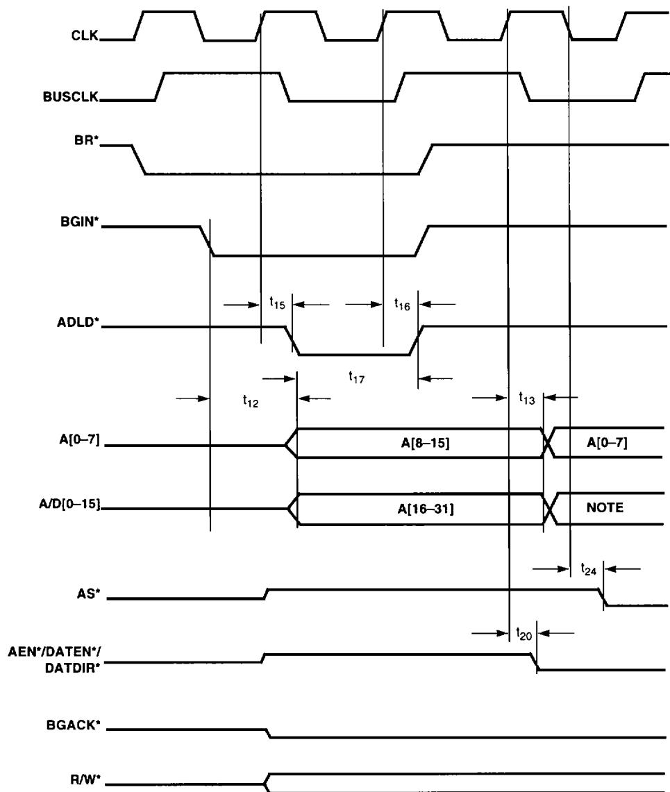
**NOTE:** In DMA Read Cycle, these pins will be tristated.
