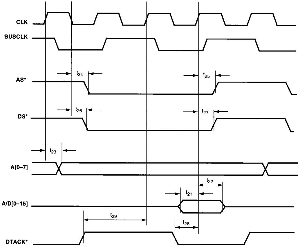
**Figure 7-6. DMA Read Cycle Timing**
