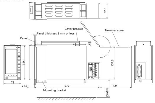
Note) The distance between other instruments and low end of PDA shall be more than 100mm.
