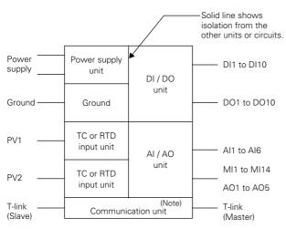
(Note) The communication unit is not isolated from the AI/AO unit when using T-link.
