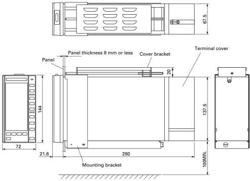
Note) The distance between other instruments and low end of PDA shall be more than 100mm.
