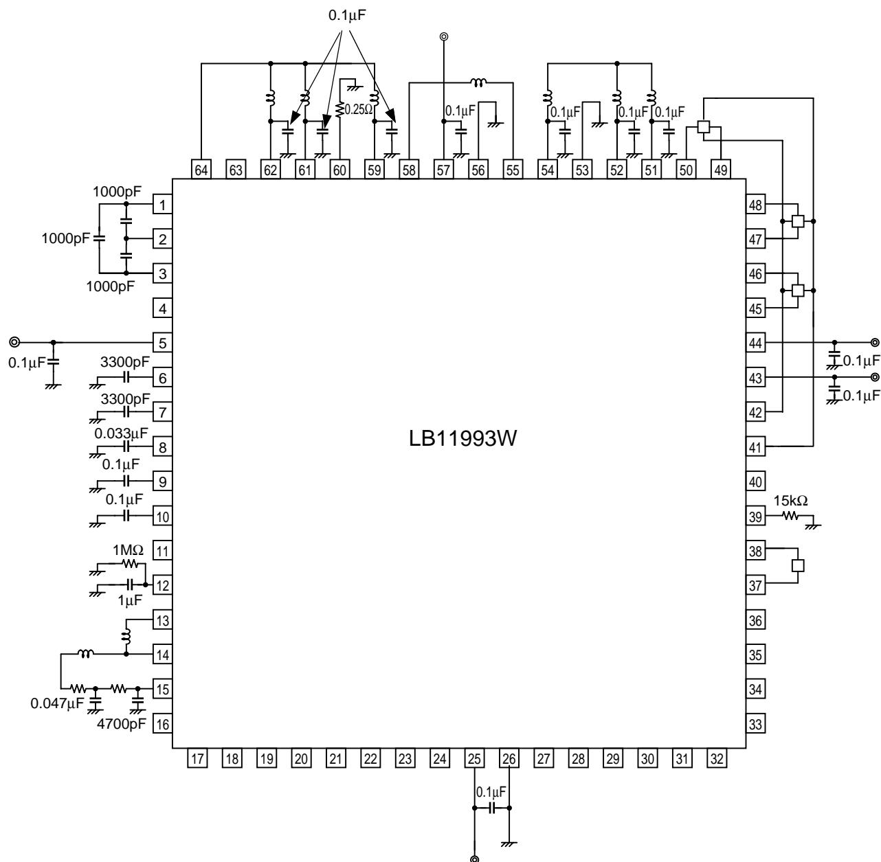
Note: The external constant is reference and may vary depending on the motor to be connected.
