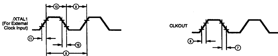
(a) XTAL1 Timing for External Clock Input
